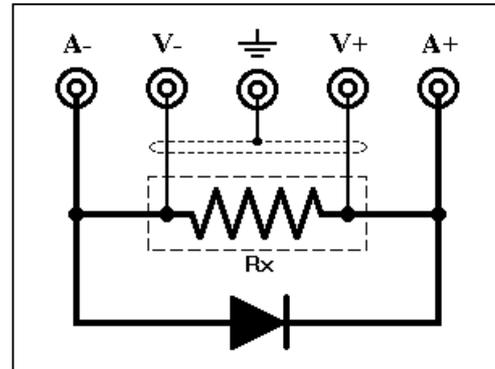
Fig. 4 Connection diagram of the protection diode in parallel with an strongly inductive element. Note the direction of insertion of the diode.
