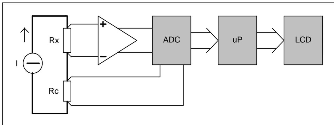
Fig. 1 Block diagram of the microohmmeter 20046 and the four-wire measurement.
