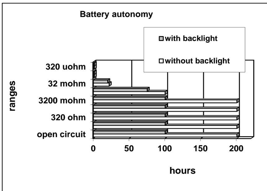
Tab. 2 Graph representing the battery autonomy in function of the selected range and the status of the backlight.
