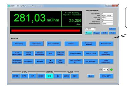
Main program window from which you can select the desired range, the sampling rate, the filter size, the secondary measure and all other operating modes and the operating parameters.
