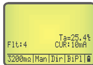
Setting the room temperature for compensated measurement.
